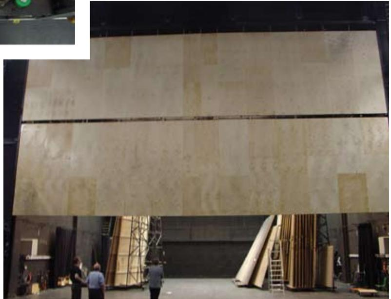
**The wagon is stored in two parts, each of which consists of two connecting sections**
