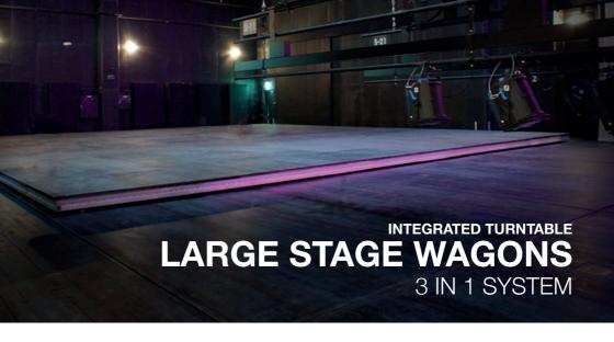
The modularity of the 3 in 1 stage wagon system enables maximum flexibility. Yesterday as a stage-sized stage wagon, today as a turntable and tomorrow for moving a car across the stage. As a stage-sized stage wagon, it can be moved from the main stage to the side stages as needed.
